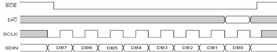
Gambar 2.22. Serial Bus Protocol-transmission of one byte.
