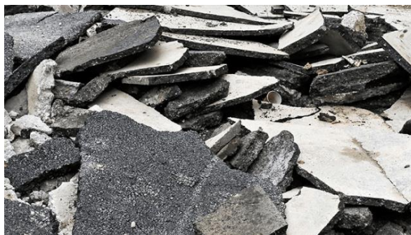
Gambar 4. 6 Reclaimed Asphalt Pavement (sumber : TheConstructor, 2020)
