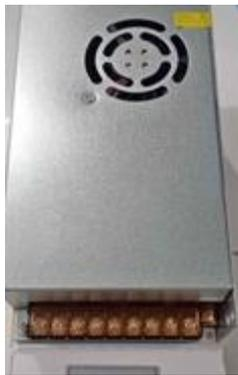
Gambar 2. 24 Power Supply 250W 24V 30A 115/230V
