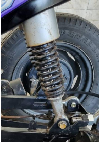
Gambar 2. 9 shockbreaker belakang suzuki shogun 110
