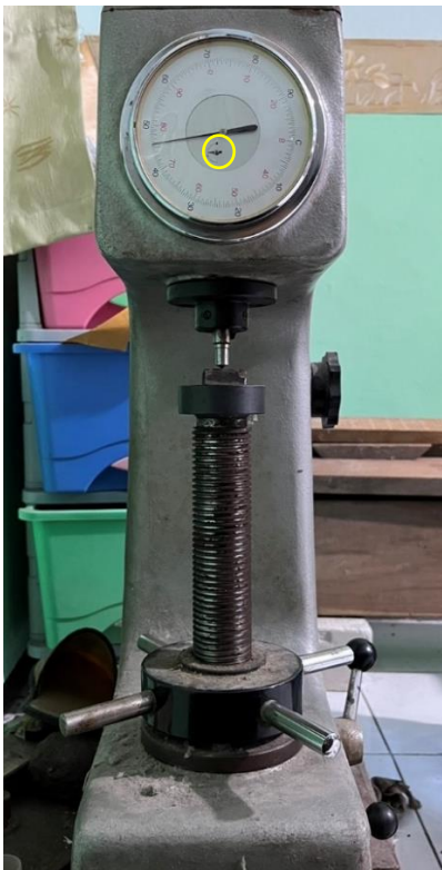
Gambar 3.8 Alat Uji Kekerasan Rockwell PT. X
