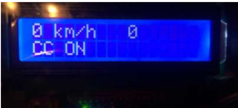
Gambar 4. 6. Tampilan LCD saat Cruise Control ON
