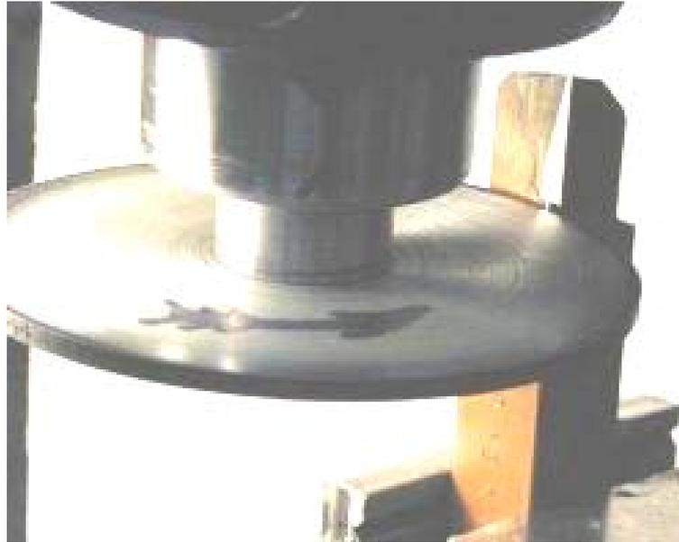
Gambar 3.7. Proses *sawing*/gergaji. <http://www.docsmachine.com>
