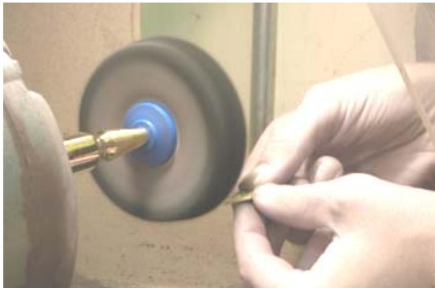
Gambar 2.6. Proses *polishing*. <http://www.docsmachine.com>
