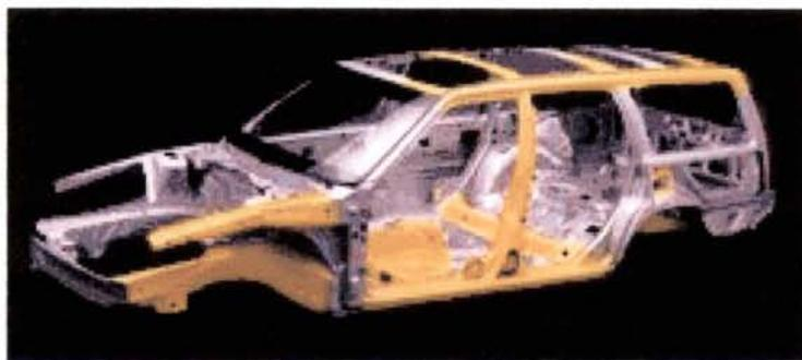
Gambar 2.3 *Monocoque Chassis*
