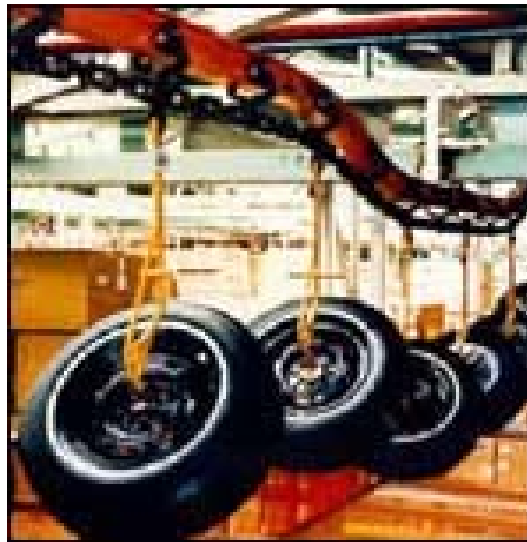
Gambar 2.5. Overhead Trolley Conveyor
