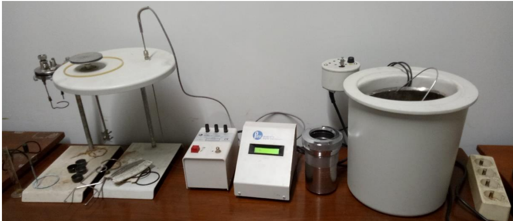
Gambar 3.6 Plain jacket bomb calorimeter
