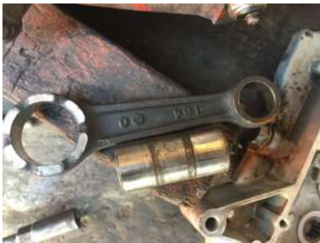
Gambar 4.12 Kondisi awal connecting rod .
