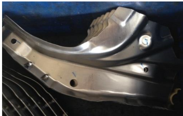
Gambar 4.12 Gambar Reinforcement Hinge
