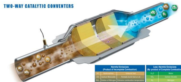
Gambar 2.7. Catalytic Converter jenis 2-way
