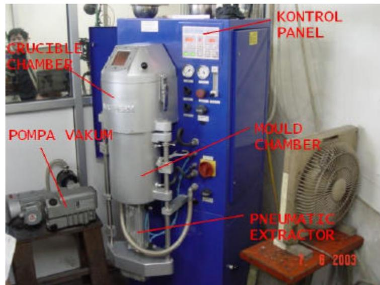
Gambar 3.12 Static Vacuum Casting Machine
