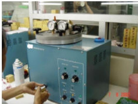
Gambar 3.5 Mesin Wax Injector
