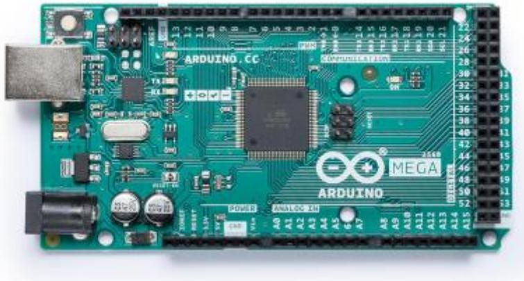
Gambar 2.2 *Arduino Mega*
