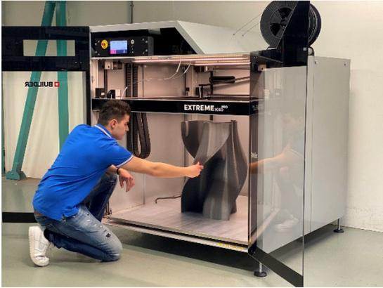
Gambar 2. 12. Industrial FDM Printer.
