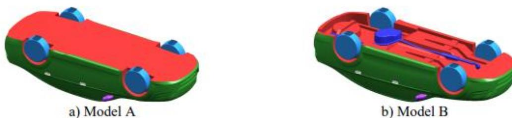
Gambar 2.14 *Flat Underbody vs Real/complex Underbody*
