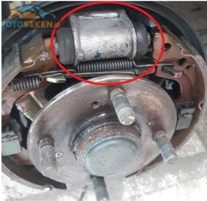
Gambar 2.17 Silinder Rem Tromol
