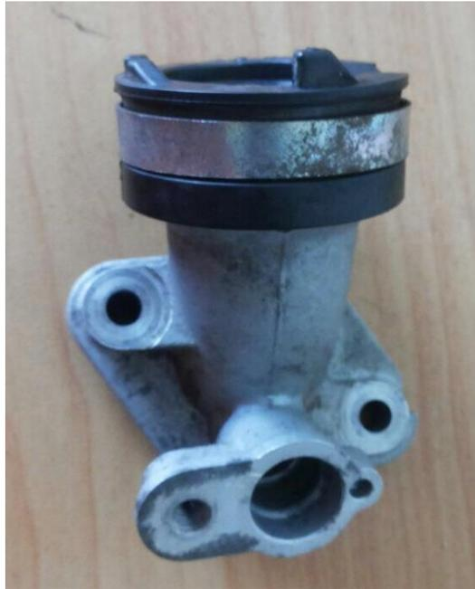
Gambar 3.15. *Intake Manifold* Standar.
