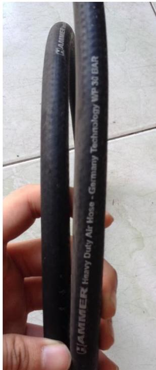
Gambar 3.13. Selang Gas *Hammer* 30 bar.
