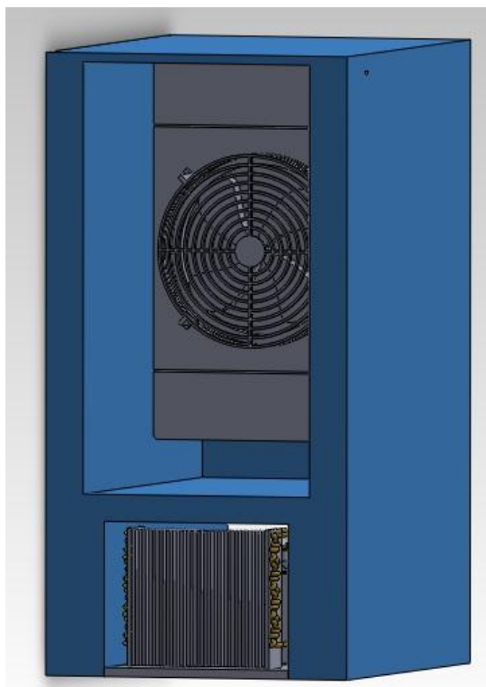
Gambar 4.14 Pendisainan Blast Chiller Kapasitas 20 Liter
